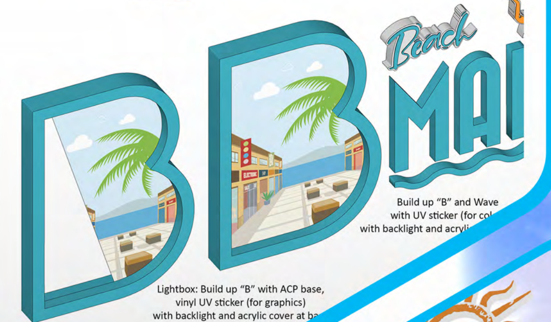
Build up Letters and Wave with UV sticker (for color) with backlight and acrylic cover at
