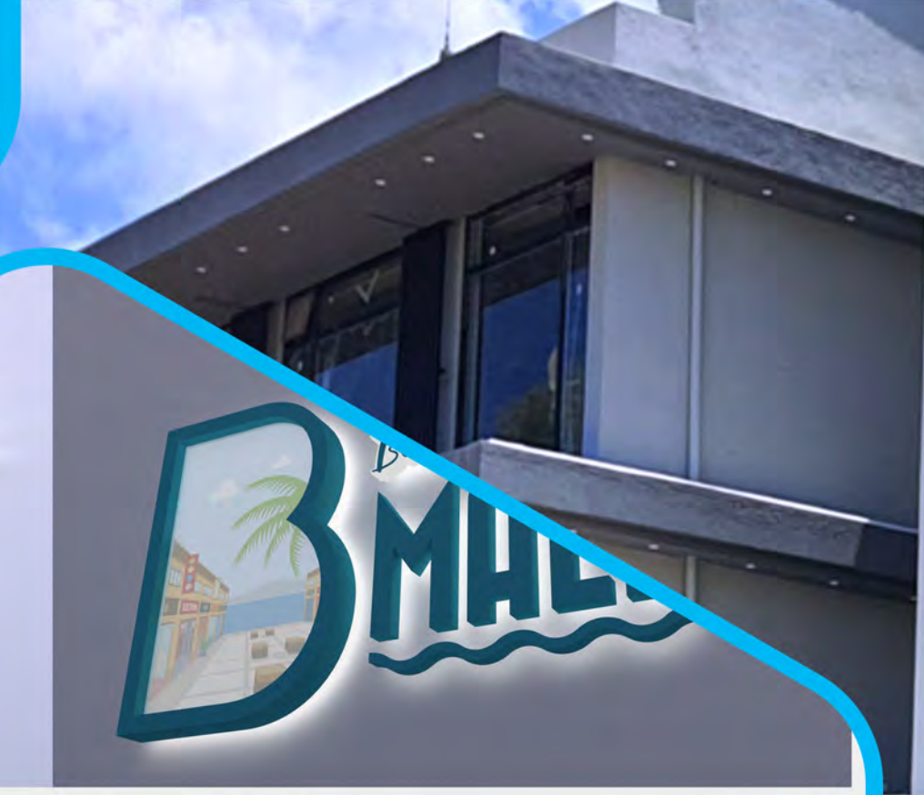
Lightbox: Build up "B" with ACP base, vinyl UV sticker (for graphics) with backlight and acrylic cover at
